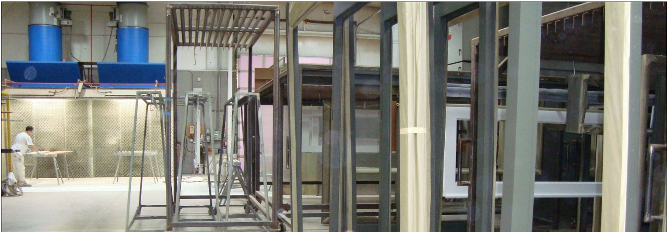
Quantum's finishing shop features drying racks surrounded by radiant heat, within an atmosphere of freshly filtered and circulated air.
