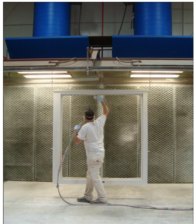
Highly qualified Quantum craftsmen operate cutting edge technology within generous shop space, excellent lighting and unlimited resources. In house finishing ensures that all glazing pockets, kerfs and mortises are sealed prior to glazing.
